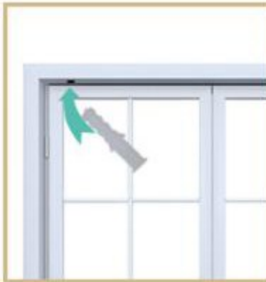
03. Input the plastic screw into the holes
